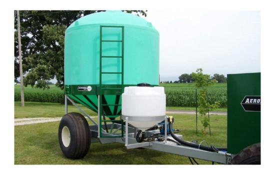
Aeromaster Water Trailers supply Aeromaster Compost Turners with the water and microbial inoculants needed to maximize process efficiency and product quality.
