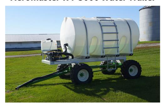
Aeromaster WT-3000 is a versatile, four-wheel 3000-gallon water tank trailer with an inoculation tank, pump, valves, and plumbing for operation with the Aeromaster PT Compost Turners.
