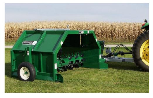
The Aeromaster PT-120 pull-type compost windrow turner is the ideal turner for sites producing up to 5,000 tons of finished compost per season (actual site capacity will vary with the length of the productive season). Its innovative design allows a single operator to aerate, blend, and add water & inoculants in a single turning pass.
