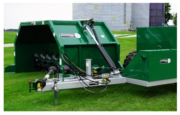
The Aeromaster PT-130 pull-type compost windrow turner is the ideal turner for sites producing up to 9,000 tons of finished compost per season (actual site capacity will vary with the length of the productive season). Its innovative design allows a single operator to aerate, blend, and add water & inoculants in a single turning pass.
